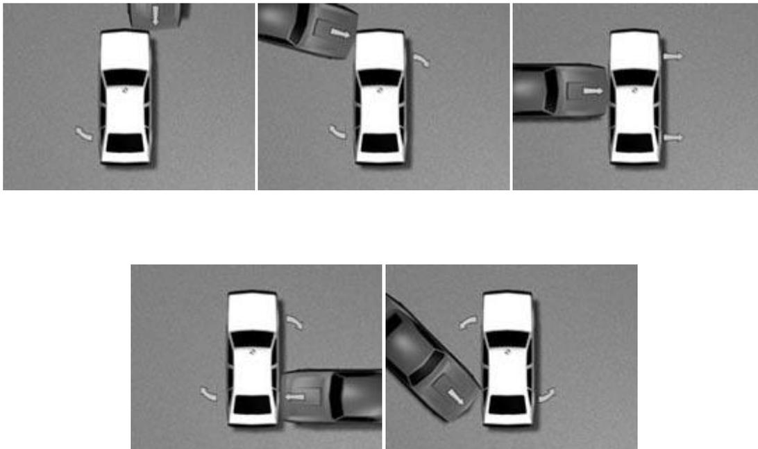
One complicating factor in occupant kinematics is vehicle rotation. Although the same principles apply in vehicles which rotate, the rotation may "change the destination" of the occupant. For instance, if the driver's direction of travel indicates secondary contact with the passenger's side of the dash, and if the vehicle is also rotating
