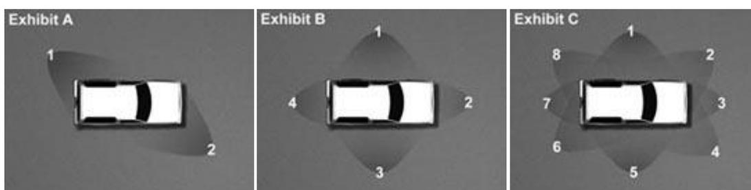
Whenever possible, a measuring device should be included in your photographs and should be used when photographing both the damaged and the undamaged areas of the vehicle. The measuring device is a useful tool to evaluate matching damage profiles. For example, let's say a Ford Escort allegedly struck the side of a BMW on the passenger's side. Once we have the measurements of the Ford's bumper height, we can compare it with the damaged
